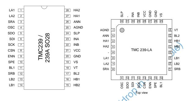
Note: Cooling plane on -LA type should be connected to GND or left open.
