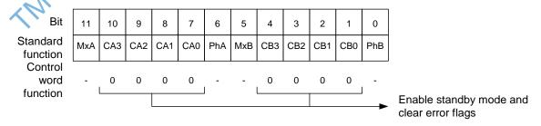
Programming current value "0000" for both coils at a time clears the overcurrent flags and switches the TMC239 into a low current standby mode with coils switched off.
