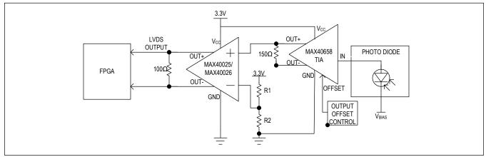
Figure 9. Single-Ended Output Receiver
