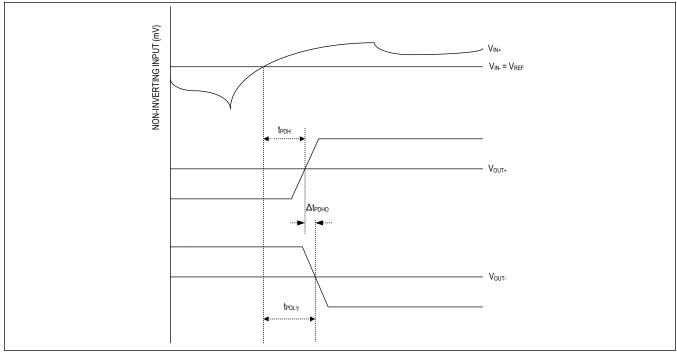
Figure 2. Propagation Delay
