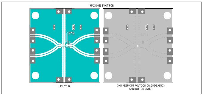
Figure 7. Layout Guidelines—Ground Keep-Out to Avoid Stubs.
