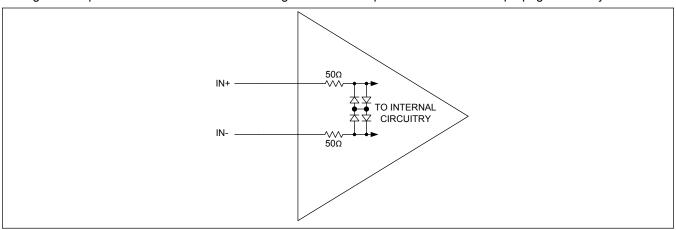
Figure 6. Input Stage Circuitry
