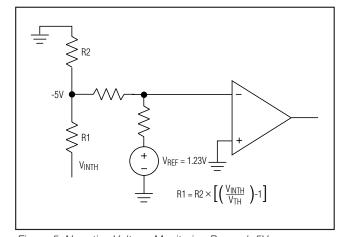
Figure 5. Negative Voltage Monitoring Beyond -5V
