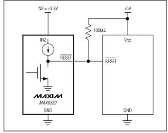
Figure 3. Interfacing to Different Logic Supply Voltage
