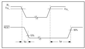
Figure 2. RESET Output Timing Diagram
