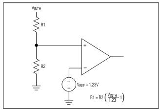
Figure 4. Setting the Auxiliary Monitor
