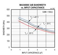
$(V_{CC} = +3.3V, C_{IN} = 0.5pF (MAX40660), C_{IN} = 8pF (MAX40661), T_{A} = +25°C; unless otherwise noted.)$
