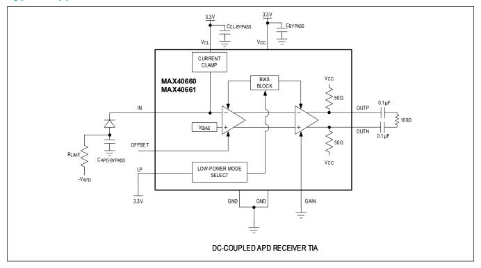
The APD's cathode is connected to to the TIA's input, and the anode is connected to the negative bias voltage through a resistor. Incident light pulses cause current to flow from the IN pin and into the APD. This input current also flows through an internal resistor to create a voltage, which is then amplified by the second stage to create a differential output signal that can drive a high-speed ADC or comparator.
