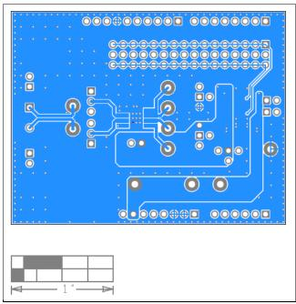
MAX33074E Shield PCB Layout—Bottom Silkscreen
