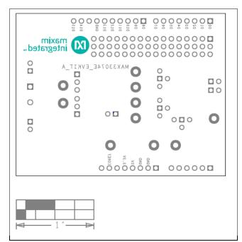
MAX33074E Shield PCB Layout—Bottom Layer
