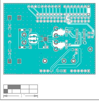
MAX33074E Shield PCB Layout—Top Layer
