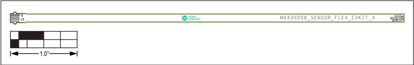
MAX30208 EV Kit Sensor Flex PCB Layout—Silk Top
