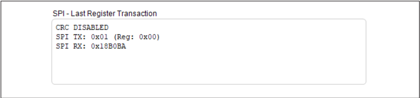
Figure 4. SPI Read Transaction with CRC Disabled
