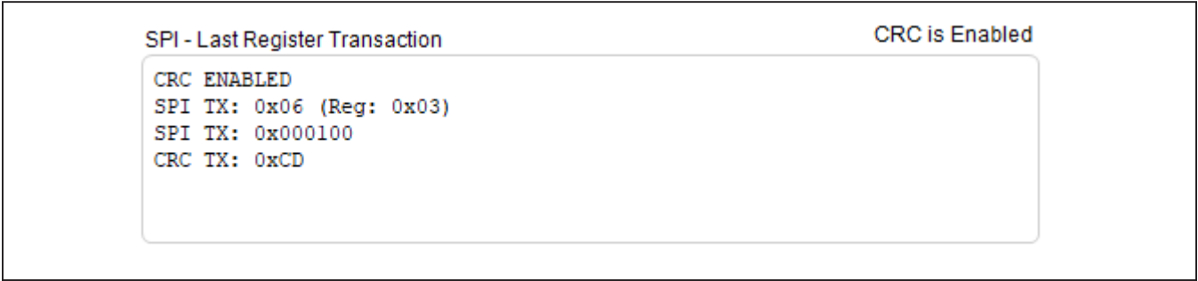
Figure 6. SPI Write Transaction with CRC Enabled
