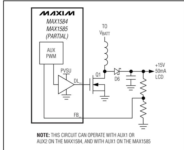
Figure 5. +15V LCD Bias with Basic Boost Topology
