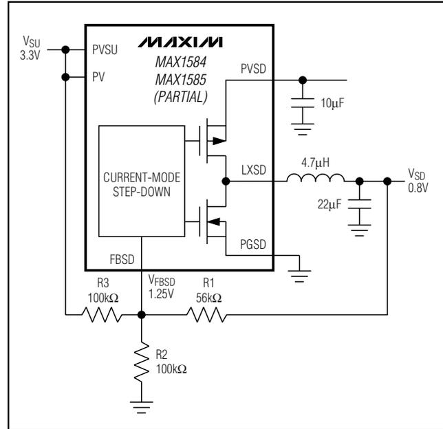
Figure 16. Setting PVSD for Outputs Below 1.25V
