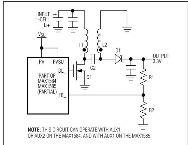
Figure 11. SEPIC Converter for Additional Boost-Buck Channel
