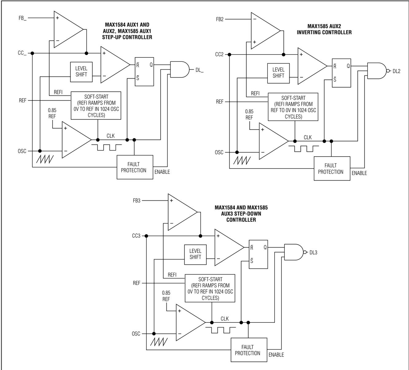
Figure 3. AUX Controller Functional Diagrams
