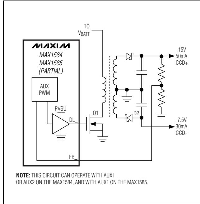
Figure 7. +15V and -7.5V CCD Bias with Transformer
