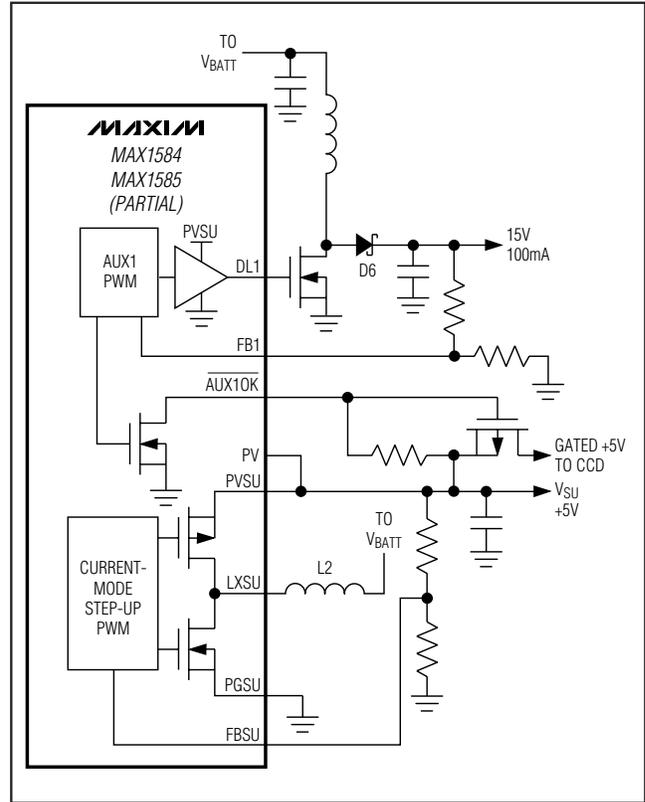
Figure 14.  $\overline{AUX1OK}$  drives an external PFET that switches 5V to the CCD only after the +15V CCD bias supply is in regulation.
