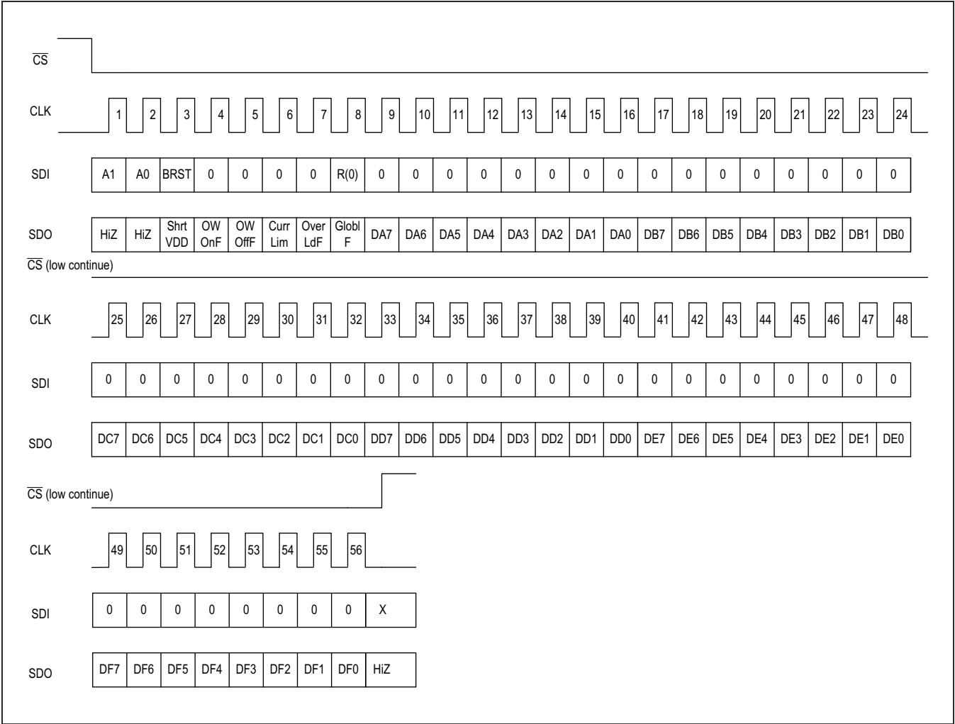
Figure 15. Addressed SPI Burst Read Command
