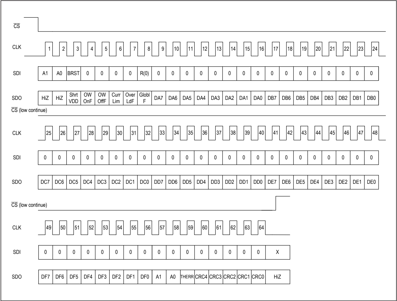
Figure 16. Addressed SPI Six Bytes Burst Read Command with CRC
