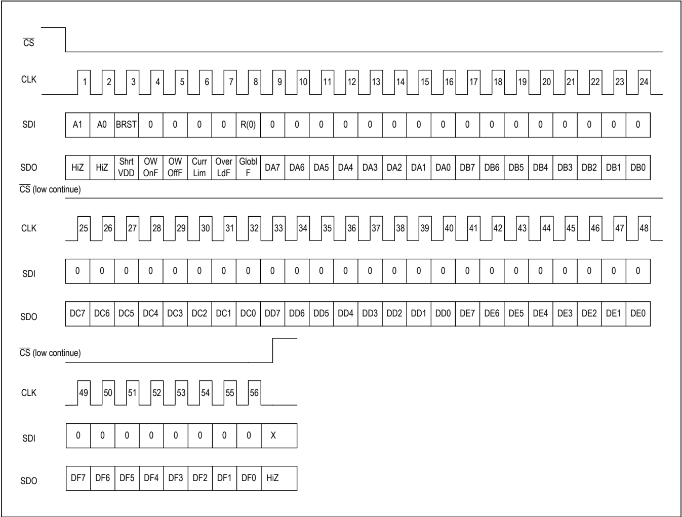
Figure 15. Addressed SPI Six Bytes Burst Read Command
