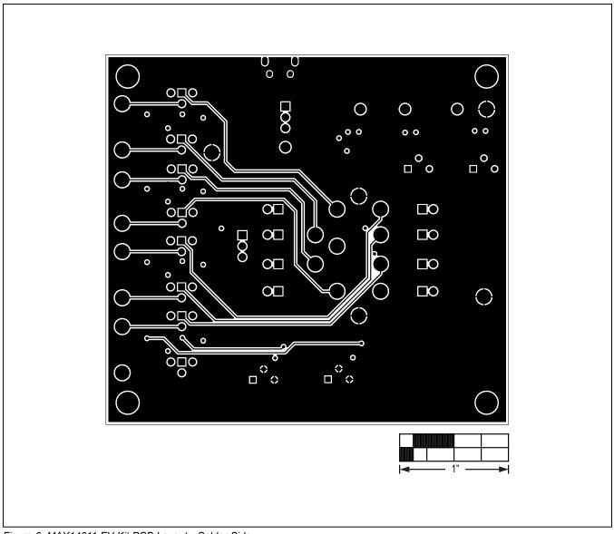
Figure 6. MAX14611 EV Kit PCB Layout—Solder Side
