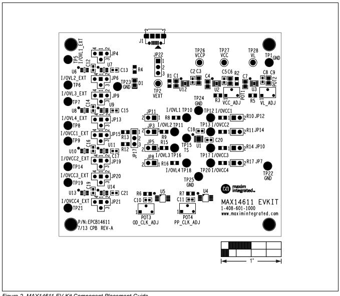
Figure 2. MAX14611 EV Kit Component Placement Guide
