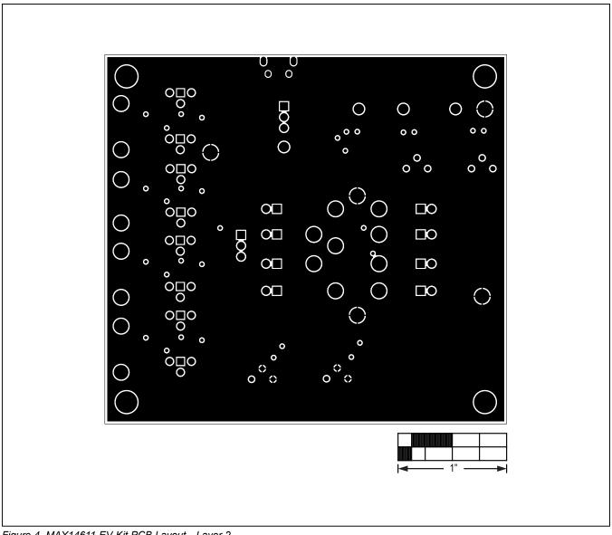
Figure 4. MAX14611 EV Kit PCB Layout—Layer 2
