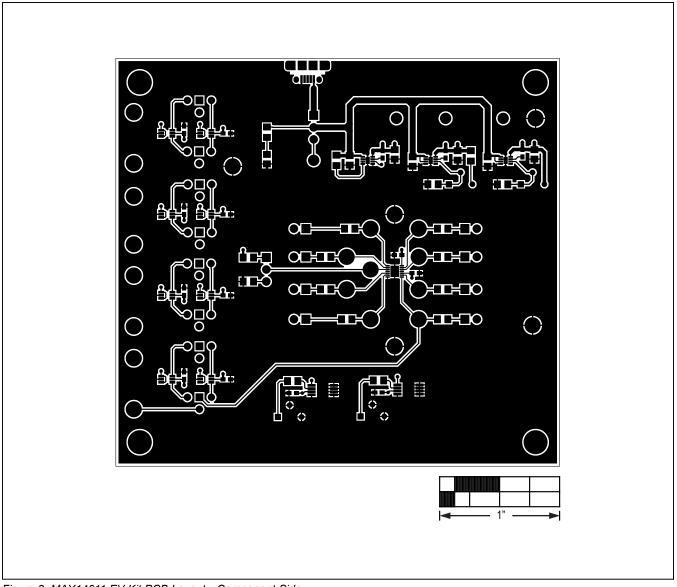
Figure 3. MAX14611 EV Kit PCB Layout—Component Side
