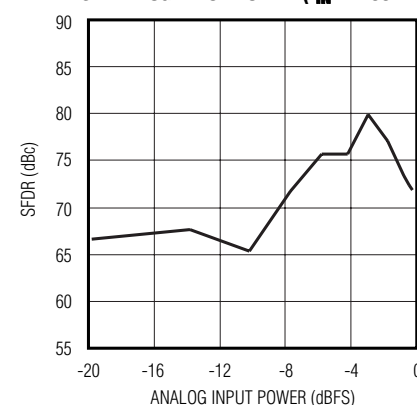
SPURIOUS-FREE DYNAMIC RANGE vs. ANALOG INPUT POWER ( f_{IN} = 7.53MHz )
