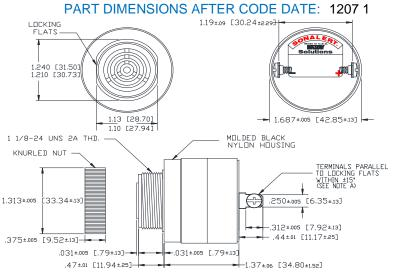
NOTE A: TERMINALS-.032 BRASS TIN PLATED, TAPPED FOR #6-32 SCREW. TWO #6-32 NICKEL PLATED BRASS SCREWS INCLUDED. WILL ACCEPT 1/4' QUICK CONNECT. NOTE B: MOUNTING- REMOVE BLACK PLASTIC NUT AND INSERT THREADED FRONT THREUGH 125' HOLE PUNCHED IN PANEL, IF DRIENTATION IS NEEDED, NOTE LOCKING FLATS ON DRAWING. SCREW NUT BACK ON. DO NOT OVERTIGHTEN.
