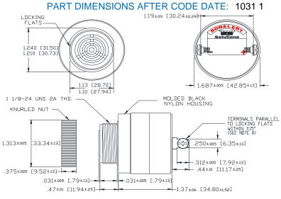
NOTE A: TERMINALS-.032 BRASS TIN PLATED, TAPPED FOR #6-32 SCREW. TVOI #6-32 NICKEL PLATED BRASS SCREWS INCLUDED. WILL ACCEPT 1/4' QUICK CONNECT. NOTE B: MOUNTING- REMOVE BLACK PLASTIC NUT AND INSERT THREADED FRONT THROUGH 1.25' HOLE PUNCHED IN PANEL, IF DRIENTATION IS NEEDED, NOTE LOCKING FLATS ON DRAWING, SCREW NUT BACK ON. DO NOT OVERTIGHTEN.
