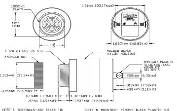
NOTE A TERMINALS-032 BRASS TIN PLATED, TAPPED FOR #6-32 SCREW, TWO #6-32 NICKEL PLATED BRASS SCREWS INCLUDED, WILL ACCEPT 1/4' QUICK CONNECT. NDTE B: MOUNTING- REMOVE BLACK PLASTIC NUT AND INSERT THREADED FRONT THROUGH 1.25' HOLE PUNCHED IN PANEL, IF DRIENTATION IS NEEDED, NOTE LOCKING FLATS ON DRAVING, SCREW NUT BACK ON. DD NOT OVERTIGHTEN.
