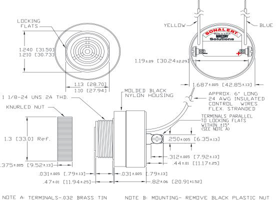
PLATED, TAPPED FOR #6-32 SCREW. TWO #6-32 NICKEL PLATED BRASS SCREWS INCLUDED. WILL ACCEPT 1/4" QUICK CONNECT.
