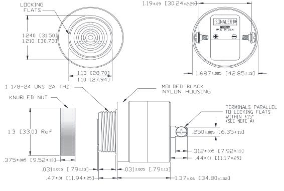
NOTE A: TERMINALS-.032 BRASS TIN PLATED, TAPPED FOR #6-32 SCREW. TWO #6-32 NICKEL PLATED BRASS SCREWS INCLUDED. WILL ACCEPT 1/4" QUICK CONNECT.
