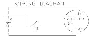
IF S1 IS OPEN, UNIT IS CONTINUOUS IF S1 IS CLOSED, UNIT IS PULSATING
