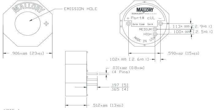
NOTE A: TERMINALS - .031" DIA. NICKEL/TIN COATED BRASS. NOTE B:
