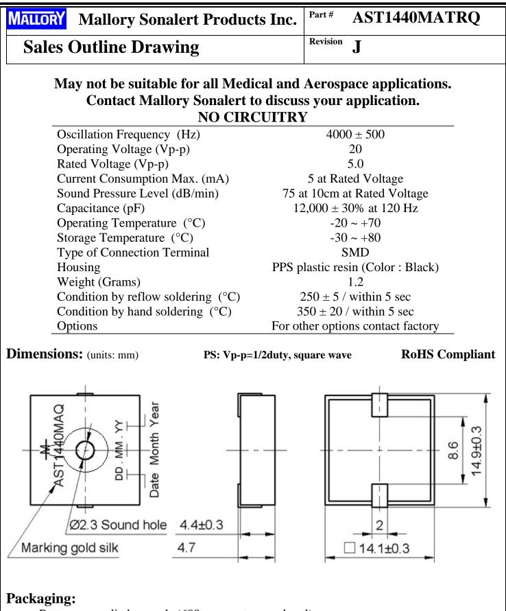
Parts are supplied on reels (600 pcs per tape and reel). Units come with wash label and are appropriate for aqueous wash.
