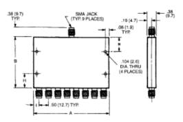
All dimensions are  $\pm$  .020, except mounting hole diameters ( $\pm$  .005) and mounting hole location ( $\pm$  .010) .
