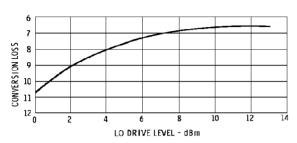
F<sub>R</sub> = 1000 MHz F<sub>L</sub> = 1020 MHz F<sub>1</sub> = 20 MHz
