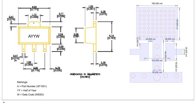
Reference Application Note M538 for lead-free solder reflow recommendations. Meets JEDEC moisture sensitivity level 1 requirements. Plating is 100% matte tin plating over copper
