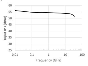
13. Input IP3 were measured using connectorized evaluation board. The RF input power was 14 dBm per tone with spacing of 1 MHz.
