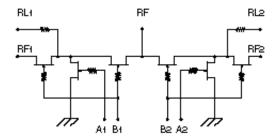
Loss changes 0.0025 dB/°C (From -55°C to +85°C) For relective operation RL1/RL2 are unconnected. For absorptive operation RL1 connects to RF1 and RL2 connects to RF2.
