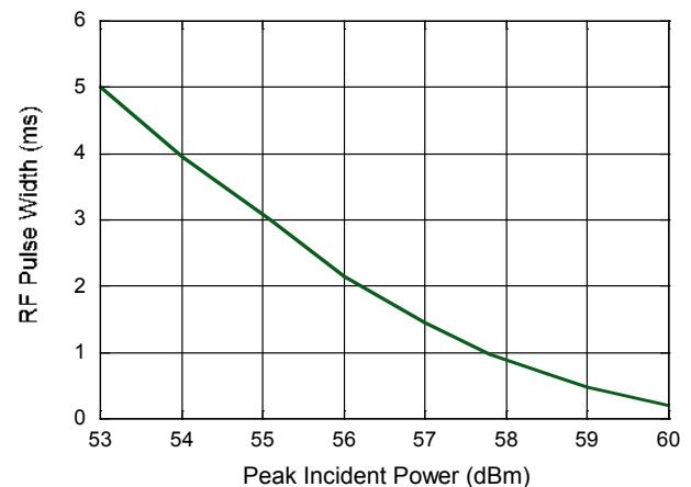
Pulse Width vs. Peak Input Power @ +85^\circ\text{C} (10% Duty Cycle, 1.3 GHz)
