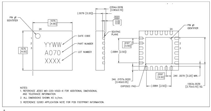
Reference Application Note S2083 for lead-free solder reflow recommendations. Meets JEDEC moisture sensitivity level 1 requirements. Plating is 100% matte tin over copper.
