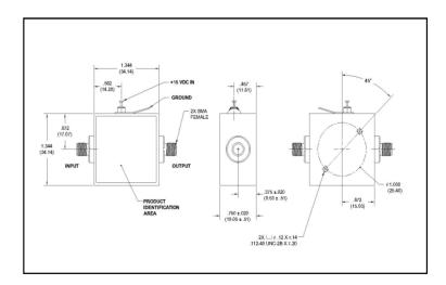
\* Dimensions are inches (millimeters) ±0.015 (0.38) unless otherwise specified.
