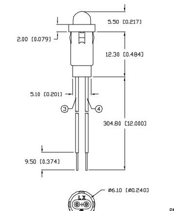
PANEL HOLE: Ø0.250" PANEL THICKNESS: 0.030" MIN.
