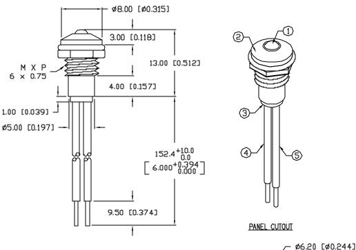
ELECTRO-OPTICAL CHARACTERISTICS TA=25°C  $V_{f} = 12V$ PARAMETER MIN TYP MAX UNITS TEST COND PEAK WAVELENGTH 635 nm FORWARD VOLTAGE 12.0 ٧f 14.0 REVERSE VOLTAGE 5.0 I<sub>r</sub>=100μA AXIAL INTENSITY 15  $V_f = 12V$ mcd VIEWING ANGLE 2x theta EMITTED COLOR: RED EPOXY LENS FINISH: RED DIFFUSED
