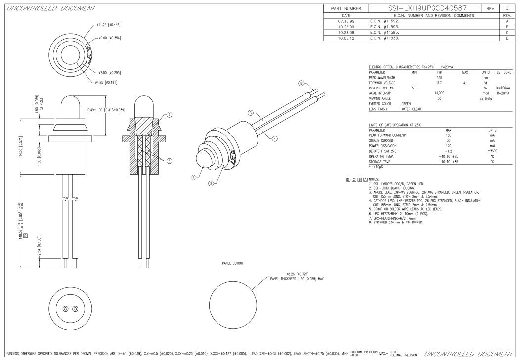
TO DECIMAL PRECISION ARE:  $x=\pm1$  (±0.039),  $x.x=\pm0.5$  (±0.020),  $x.xx=\pm0.25$  (±0.010),  $x.xxx=\pm0.127$  (±0.005). LEAD SIZE=±0.05 (±0.020), LEAD SIZE=±0.05 (±0.030). MIN=  $-\frac{1}{0.000}$  MAX.=  $-\frac{1}{$
