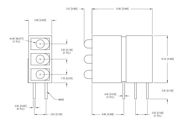
\*UNLESS OTHERWISE SPECIFIED TOLERANCES PER DECIMAL PRECISION ARE: X=±1 (±0.039), XX=±0.5 (±0.020), XXX=±0.25 (±0.010), XXXX=±0.127 (±0.005). LEAD SIZE=±0.05 (±0.002), LEAD LENGTH=±0.75 (±0.030). MIN=  $\frac{+0.00}{-0.00}$  MAX.=  $\frac{+0.00}{-0.00}$  MAX
