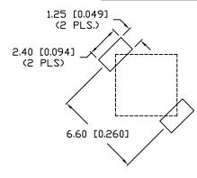
\*UNLESS OTHERWISE SPECIFIED TOLERANCES PER DECIMAL PRECISION ARE: X=±1 (±0.039), X.XX=±0.5 (±0.020), X.XXX=±0.127 (±0.005). LEAD SIZE=±0.05 (±0.002), LEAD LENGTH=±0.75 (±0.030). MIN=+DECIMAL PRECISION MAX.= +0.00 (±0.005). LEAD SIZE=±0.05 (±0.002), LEAD LENGTH=±0.75 (±0.030). MIN=+DECIMAL PRECISION MAX.= +0.00 (±0.005).
