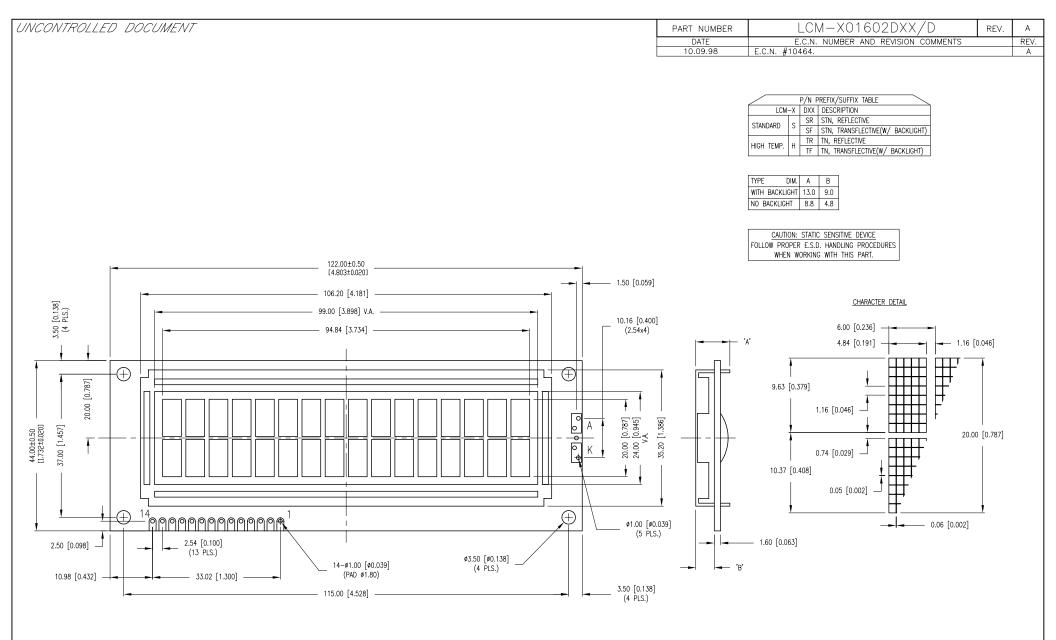
\*UNLESS OTHERWISE SPECIFIED TOLERANCES PER DECIMAL PRECISION ARE: X=±1 (±0.039), X.X=±0.5 (±0.020), X.XX=±0.25 (±0.010), X.XXX=±0.127 (±0.005). LEAD SIZE=±0.05 (±0.002), LEAD LENGTH=±0.75 (±0.030). MIN= +DECIMAL PRECISION MAX.= +D.00
