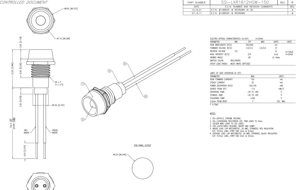
\*UNLESS OTHERWISE SPECIFIED TOLERANCES PER DECIMAL PRECISION ARE:  $x=\pm1$  (±0.039),  $x.x=\pm0.5$  (±0.020),  $x.xx=\pm0.25$  (±0.010),  $x.xx=\pm0.127$  (±0.005). LEAD SIZE=±0.05 (±0.002), LEAD LENGTH=±0.75 (±0.030). MIN=  $\frac{+0.001}{-0.000}$  MAX.=  $\frac{+0.001}{-0.0$
