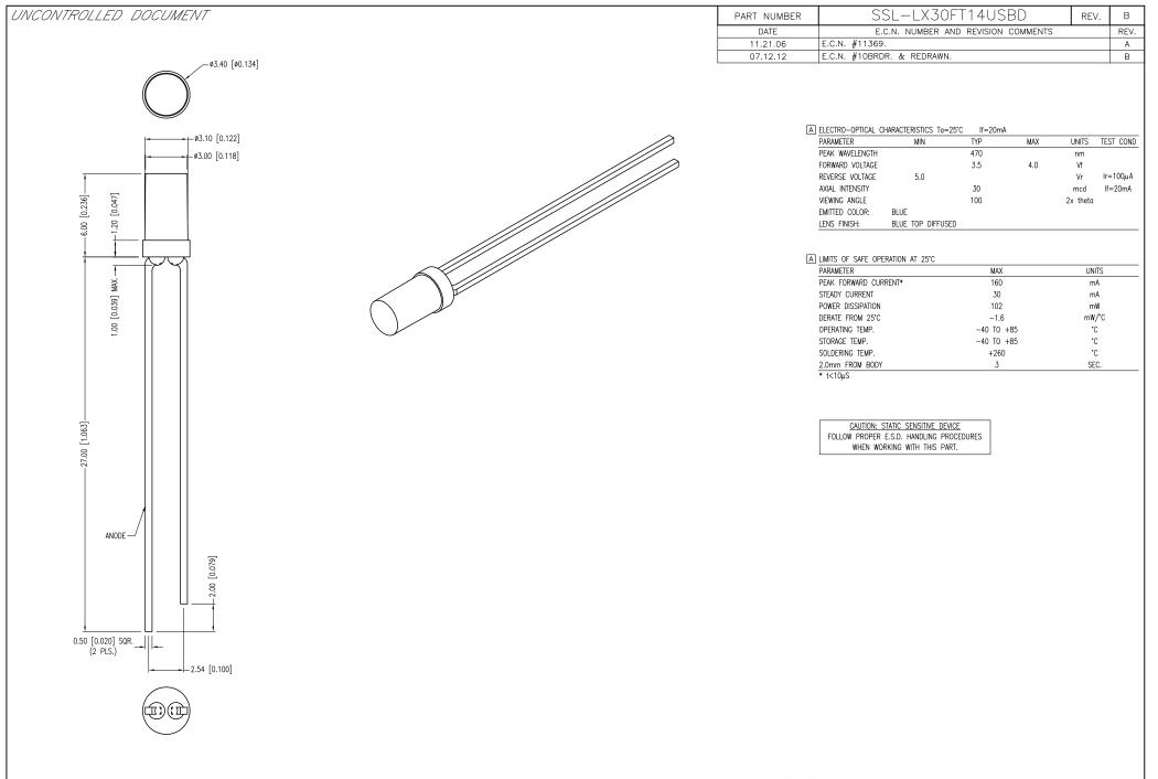
\*UNLESS OTHERWISE SPECIFIED TOLERANCES PER DECIMAL PRECISION ARE: X=±1 (±0.039), X.X=±0.5 (±0.020), X.XX=±0.25 (±0.010), X.XXX=±0.127 (±0.005). LEAD SIZE=±0.05 (±0.002), LEAD LENGTH=±0.75 (±0.030). MIN= +DECIMAL PRECISION MAX.= +0.00 -0.00 MAX.= +DECIMAL PRECISION ARE: X=±1 (±0.039), X.X=±0.5 (±0.020), X.XX=±0.25 (±0.010), X.XXX=±0.127 (±0.005). LEAD SIZE=±0.05 (±0.002), LEAD LENGTH=±0.75 (±0.030). MIN= +DECIMAL PRECISION MAX.= +0.00
