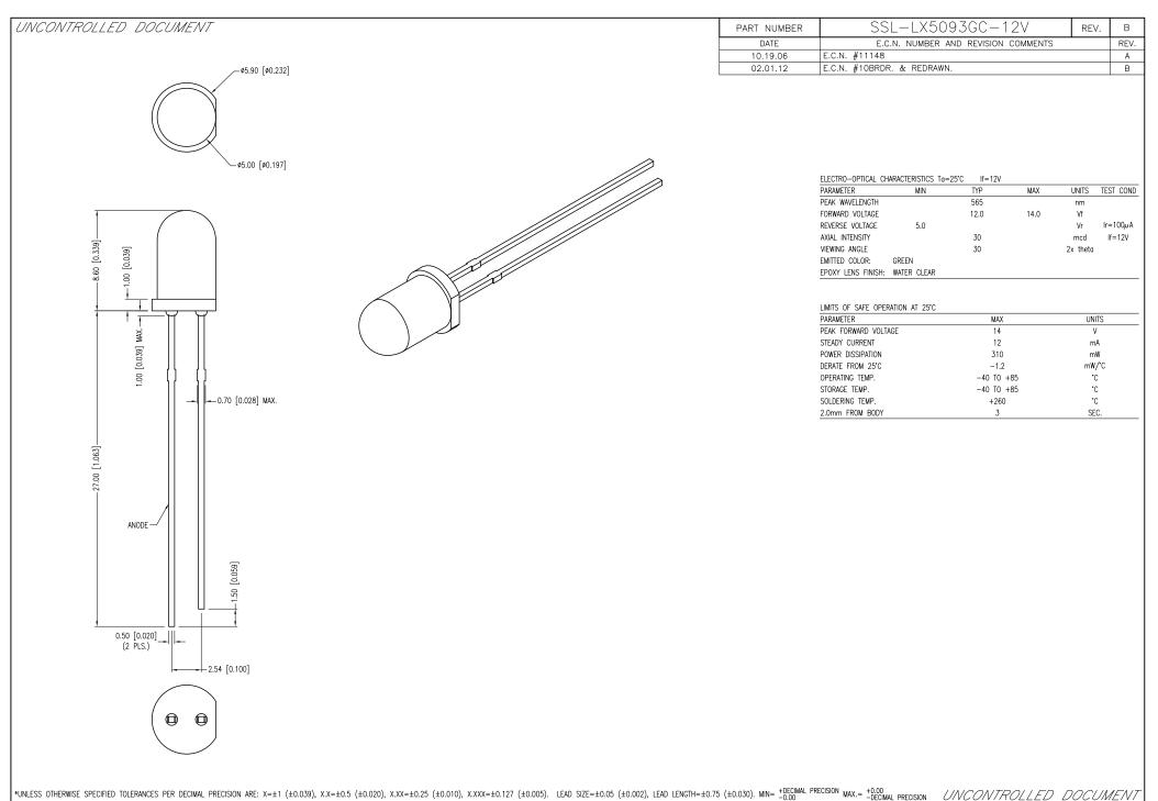
DRAWN BY: DATE: 02.01.12 AB QUASARBRITE T-5mm (T-1 3/4) 565nm GREEN LED, WATER CLEAR LENS, 12 VOLT OPERATION. 425 N. GARY AVE. CAROL STREAM, IL 60188-4900 PAGE: 1 OF CHKD BY: ΚF 1 PHONE: +1.800.278.5666 \*\*THE SPECIFICATIONS MAY CHANGE AT ANY TIME WITHOUT NOTICE DUE TO NEW MATERIALS OR PRODUCT IMPROVEMENT.\*\* FAX: +1.630.315.2152 SCALE: NTS APRVD BY: ΚF
