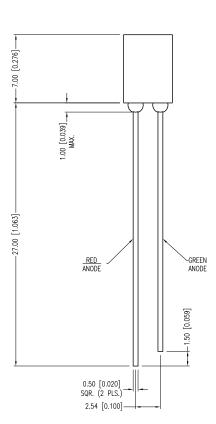
\*UNLESS OTHERWISE SPECIFIED TOLERANCES PER DECIMAL PRECISION ARE: X=±1 (±0.039), X.X=±0.5 (±0.020), X.XX=±0.25 (±0.010), X.XX=±0.127 (±0.005). LEAD SIZE=±0.05 (±0.002), LEAD LENGTH=±0.75 (±0.030). MIN =  $\frac{+0.001}{-0.001}$  MAX.=  $\frac{+0.001}{-0.001}$  MA
