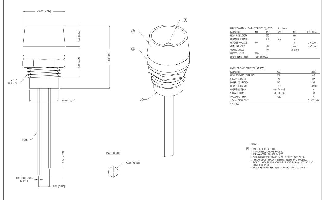
\*UNLESS OTHERWISE SPECIFIED TOLERANCES PER DECIMAL PRECISION ARE: X=±1 (±0.039), X.X=±0.5 (±0.020), X.XX=±0.25 (±0.010), X.XXX=±0.127 (±0.005). LEAD SIZE=±0.05 (±0.002), LEAD LENGTH=±0.75 (±0.030). MIN= +DECIMAL PRECISION MAX.= +0.00 -0.00 MAX.= +0.00
