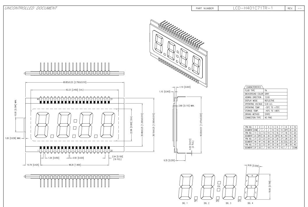
\*UNLESS OTHERWISE SPECIFIED TOLERANCES PER DECIMAL PRECISION ARE: X=±1 (±0.039), X.X=±0.5 (±0.020), X.XX=±0.25 (±0.010), X.XXX=±0.127 (±0.005). LEAD SIZE=±0.05 (±0.002), LEAD LENGTH=±0.75 (±0.030). MIN=  $^{+0.001}_{-0.00}$  MAX.=  $^{+0.00}_{-0.001}$  MAX.=  $^{+0.00}_{-0.001}$  MAX.=  $^{+0.00}_{-0.001}$  PRECISION LINICONTROLLED DOCLIMENT
