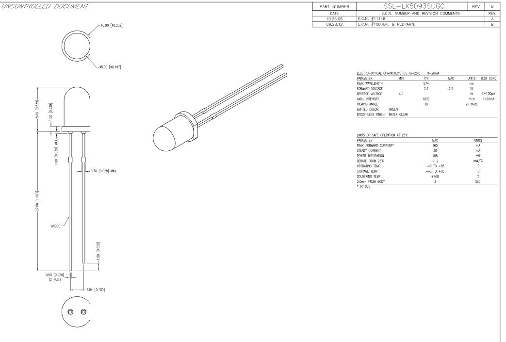
\*UNLESS OTHERWISE SPECIFIED TOLERANCES PER DECIMAL PRECISION ARE: X=±1 (±0.039), X.X=±0.5 (±0.020), X.XX=±0.25 (±0.010), X.XXX=±0.127 (±0.005). LEAD SIZE=±0.05 (±0.002), LEAD LENGTH=±0.75 (±0.030). MIN= +DECIMAL PRECISION MAX.= +0.00
