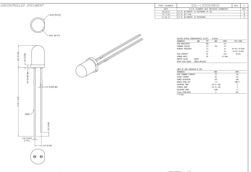
\*UNLESS OTHERWISE SPECIFIED TOLERANCES PER DECIMAL PRECISION ARE: X=±1 (±0.039), X.X=±0.5 (±0.020), X.XX=±0.25 (±0.010), X.XXX=±0.127 (±0.005). LEAD SIZE=±0.05 (±0.002), LEAD LENGTH=±0.75 (±0.030). MIN =  $^{+0.00}_{-0.00}$  MAX.=  $^{+0.00}_{-0.00}$  UNCONTROLLED DOCUMENT
