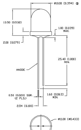
UNLESS OTHERWISE SPECIFIED TOLERANCE IS ±.25mm (±0.010")
