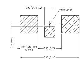
\*UNLESS OTHERWISE SPECIFIED TOLERANCES PER DECIMAL PRECISION ARE: X=±1 (±0.039), X.X=±0.5 (±0.020), X.XX=±0.25 (±0.010), X.XXX=±0.127 (±0.005). LEAD SIZE=±0.05 (±0.020), LEAD LENGTH=±0.75 (±0.030). MIN =  $\frac{+DECIMAL}{-0.00}$  MAX.=  $\frac{+0.00}{-0.00}$  MAX.=  $\frac{+0.00}{-0.0$
