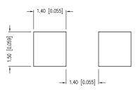
\*UNLESS OTHERWISE SPECIFIED TOLERANCES PER DECIMAL PRECISION ARE: X=±1 (±0.039), X.X=±0.5 (±0.020), X.XX=±0.25 (±0.010), X.XXX=±0.127 (±0.005). LEAD SIZE=±0.05 (±0.002), LEAD LENGTH=±0.75 (±0.030). MIN= +DECIMAL PRECISION MAX.= +0.00 (±0.002), MIN= +0.000 (±0.002
