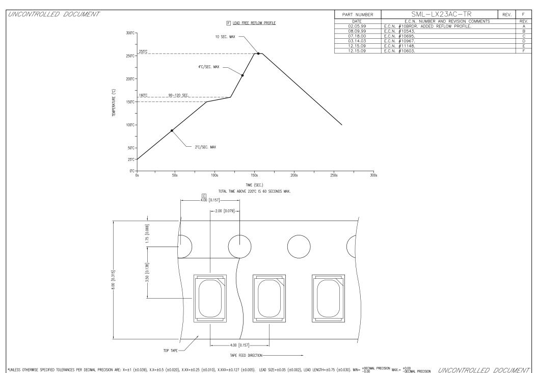
UNCONTROLLED DOCUMENT DATE: 04.05.11 DRAWN BY: AΒ 290 E. HELEN ROAD 2mm x 3mm SURFACE MOUNT WITH REFLECTOR, 610nm AMBER LED, WATER CLEAR LENS. PALATINE, IL 60067-6976 PAGE: 2 OF 2 CHKD BY: JD \*\*THE SPECIFICATIONS MAY CHANGE AT ANY TIME WITHOUT NOTICE DUE TO NEW MATERIALS OR PRODUCT IMPROVEMENT.\*\* PHONE: +1.847.359.2790 CONFIDENTIAL INFORMATION
