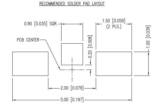
\*UNLESS OTHERWISE SPECIFIED TOLERANCES PER DECIMAL PRECISION ARE: X=±1 (±0.039), X.X=±0.5 (±0.020), X.XX=±0.25 (±0.010), X.XXX=±0.127 (±0.005). LEAD SIZE=±0.05 (±0.002), LEAD LENGTH=±0.75 (±0.030). MIN=  $^{+DECIMAL PRECISION}_{-0.00}$  MAX.=  $^{+0.00}_{-0.00}$  MAX.=  $^{+$
