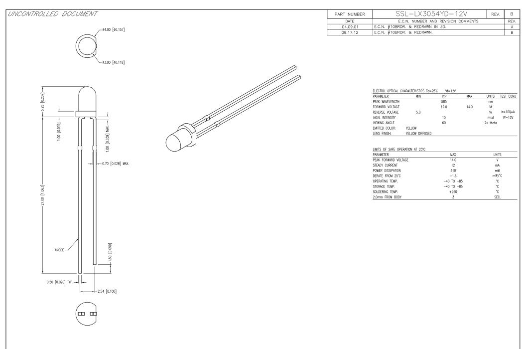
\*UNLESS OTHERWISE SPECIFIED TOLERANCES PER DECIMAL PRECISION ARE: X=±1 (±0.039), X.X=±0.5 (±0.020), X.XX=±0.25 (±0.010), X.XX=±0.127 (±0.005). LEAD SIZE=±0.05 (±0.002), LEAD LENGTH=±0.75 (±0.030). MIN= +DECIMAL PRECISION MAX.= +0.00 -DECIMAL PRECISION MAX.= +0.00 -DECIMAL PRECISION MAX.= +0.00
