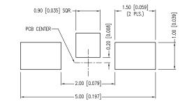
\*UNLESS OTHERWISE SPECIFIED TOLERANCES PER DECIMAL PRECISION ARE:  $x=\pm1$  (±0.039),  $x.x=\pm0.5$  (±0.020),  $x.xx=\pm0.25$  (±0.010),  $x.xxx=\pm0.127$  (±0.005). LEAD SIZE=±0.05 (±0.002), LEAD LENGTH=±0.75 (±0.030). MIN=  $\frac{+0.00}{-0.00}$  MAX.=  $\frac{+0.00}{-0.00}$
