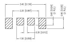
\*UNLESS OTHERWISE SPECIFIED TOLERANCES PER DECIMAL PRECISION ARE:  $x = \pm 1$  (±0.039),  $x.x = \pm 0.5$  (±0.020),  $x.xx = \pm 0.25$  (±0.010),  $x.xxx = \pm 0.25$  (±0.005). LEAD SIZE=±0.05 (±0.002), LEAD LENGTH=±0.75 (±0.030). MIN=  $\frac{+\text{DECIMAL PRECISION}}{-0.00}$  MAX.=  $\frac{+0.00}{-0.00}$
