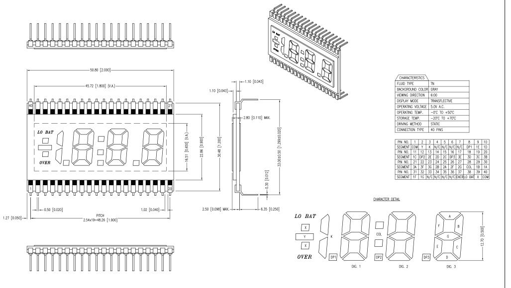
\*UNLESS OTHERWISE SPECIFIED TOLERANCES PER DECIMAL PRECISION ARE: X=±1 (±0.039), X.X=±0.5 (±0.020), X.XX=±0.25 (±0.010), X.XXX=±0.127 (±0.005). LEAD SIZE=±0.05 (±0.002), LEAD LENGTH=±0.75 (±0.030). MIN= +DECIMAL PRECISION MAX.= +0.00 -0.00
