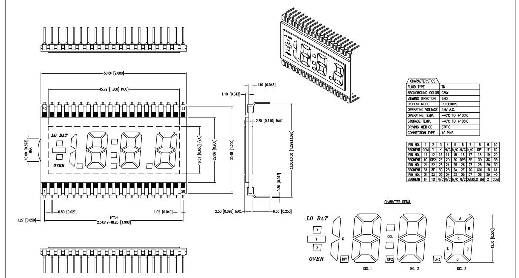
\*UNILESS OTHERWISE SPECIFIED TOLERANCES PER DECIMAL PRECISION ARE: X=±1 (±0.039), X.X=±0.5 (±0.020), X.XX=±0.25 (±0.010), X.XXX=±0.127 (±0.005). LEAD SIZE=±0.05 (±0.002), LEAD LENGTH=±0.75 (±0.030). MIN= +DECIMAL PRECISION MAX.= +0.00 MAX.= +0.00
